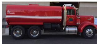
In the spring of 2015 the department purchased its second water tender to help meet the ISO requirements for a fire property protection class rating for those properties without rated fire hydrants. During ISO's examination of the department it became clear that the fire department was not capable of bringing 4,000 gallons of water to many of the tracts
