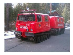
The Hagglunds snow-cat carries 13 and operates on pavement, dirt and gravel, ice and snow and can "swim" in rivers and lakes. With four driving tracks, the Hagglunds is capable of operating in the most severe winter conditions and has saved lives in the middle of winter.
